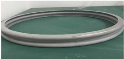
图 14 “W”形金属密封环实验件 Fig. 14 Experimental sample of the metallic W-ring
